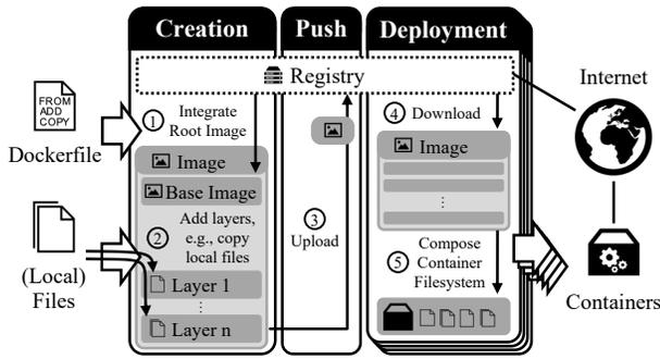
**Figure 1: The Docker Paradigm: Dockerfiles describe files and functions of images. Images are uploaded to a registry for sharing and potentially numerous administrators deploy containers based on a single image (according to [8]).**
